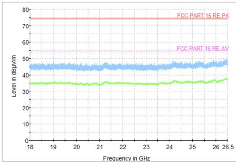
Fig.27 Radiated Spurious Emission (All Channels, 18 GHz-26.5 GHz), LE 1M
