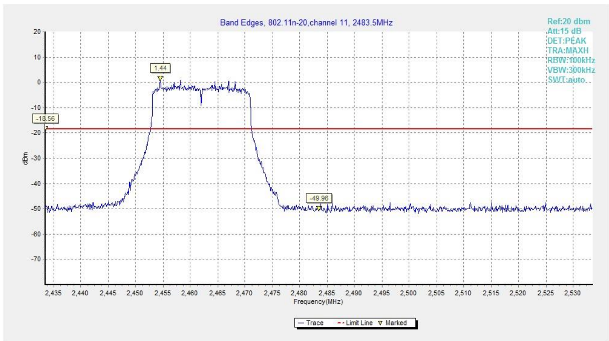
Fig.A.5.6 Band Edges (802.11n-HT20, Ch 11)
