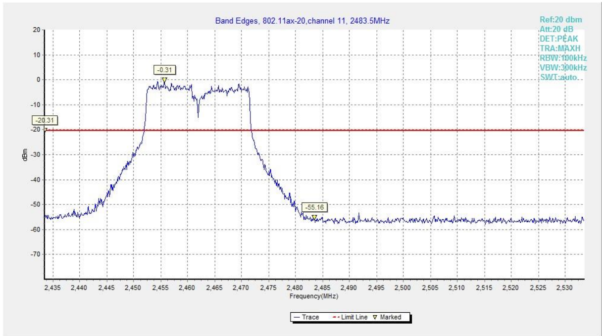
Fig.A.5.10 Band Edges (802.11ax-HE20, Ch 11)
