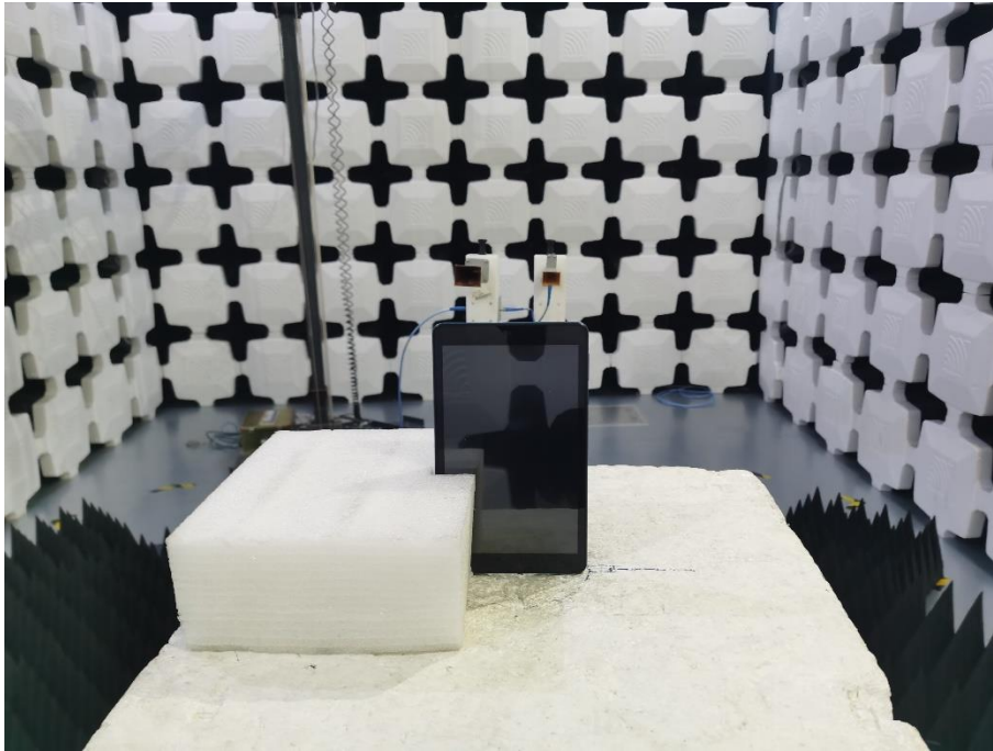
17. Radiated Emissions (Part 15C, 26.5GHz -40GHz)
