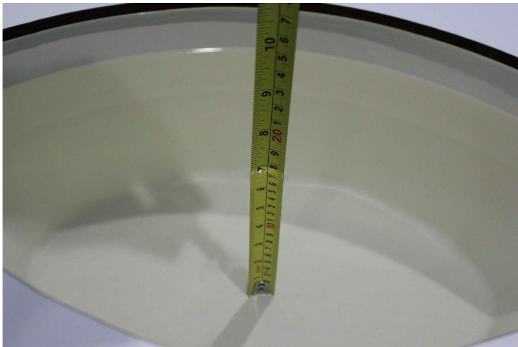
Picture 7-2: Liquid depth in the Flat Phantom(5GHz)
