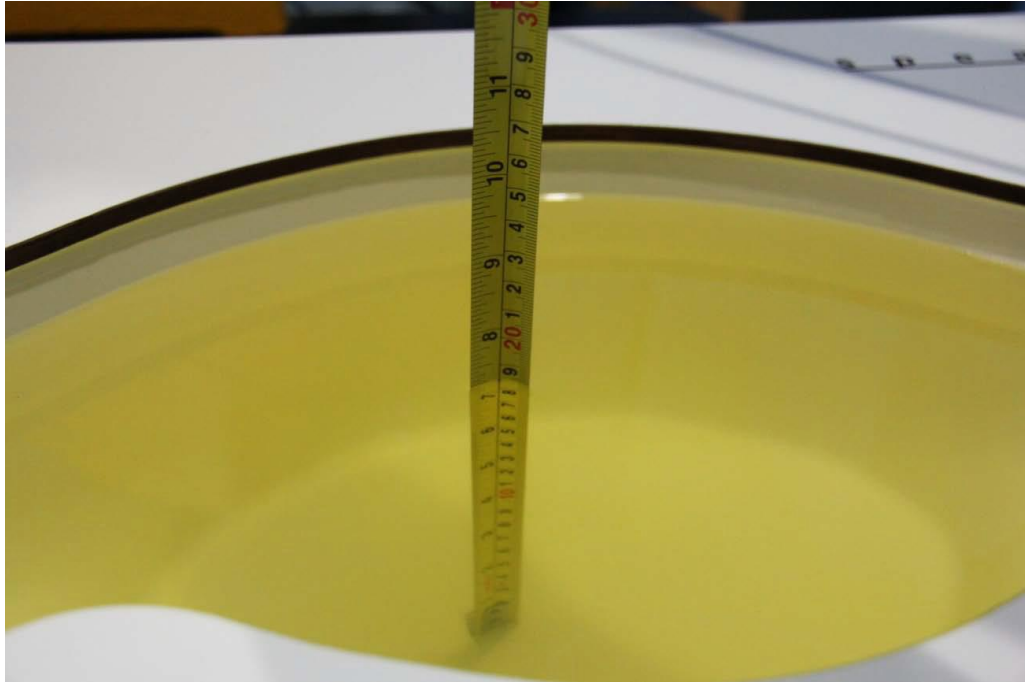
Picture 7-1: Liquid depth in the Flat Phantom(2450MHz)
