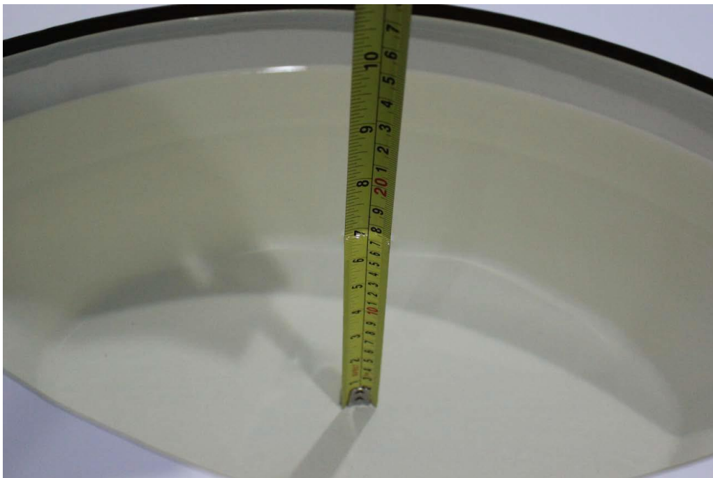
Picture 7-2: Liquid depth in the Flat Phantom(5GHz)
