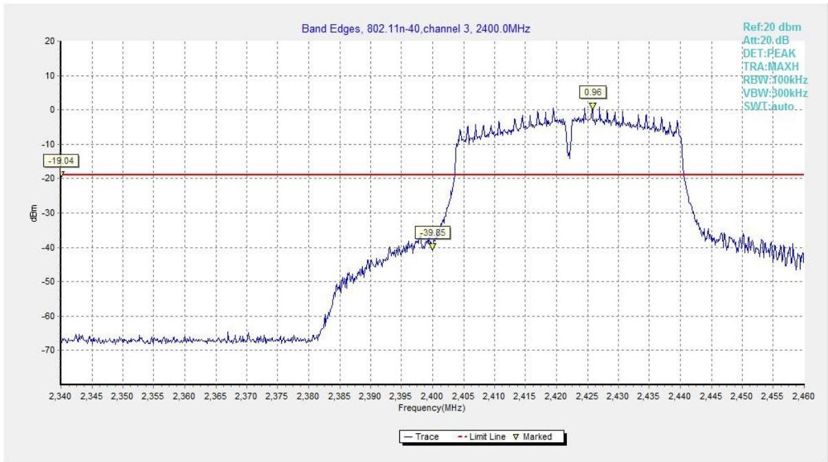
Fig.31 Band Edges (802.11n HT40, CH 3)
