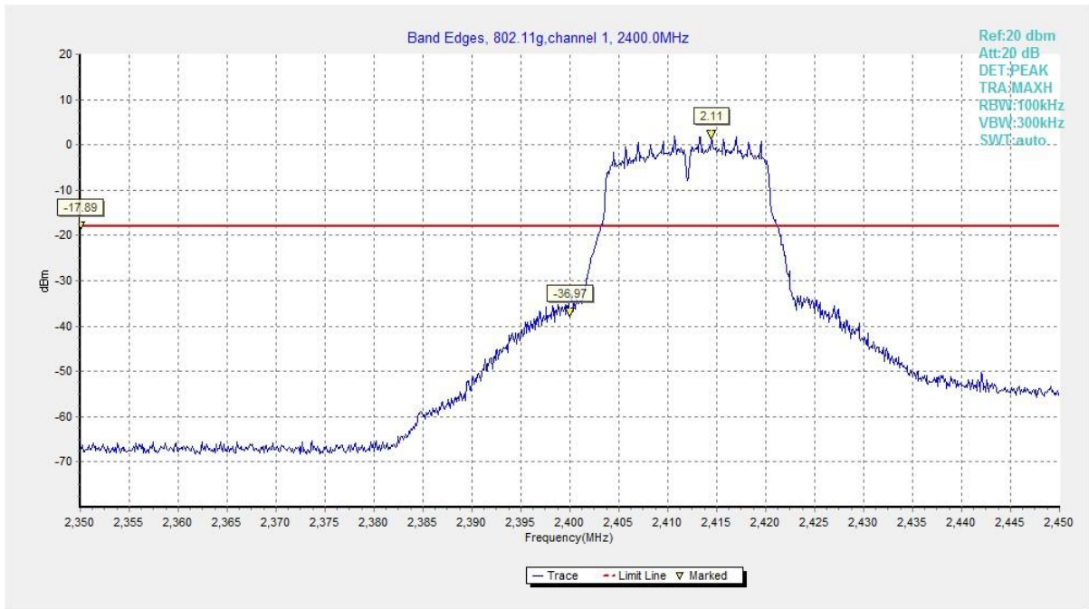
Fig.27 Band Edges (802.11g, CH 1)
