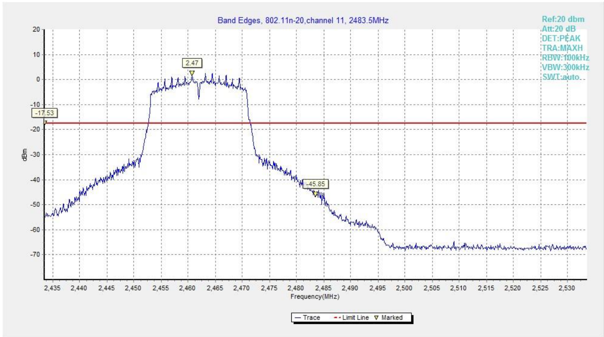
Fig.30 Band Edges (802.11n HT20, CH 11)
