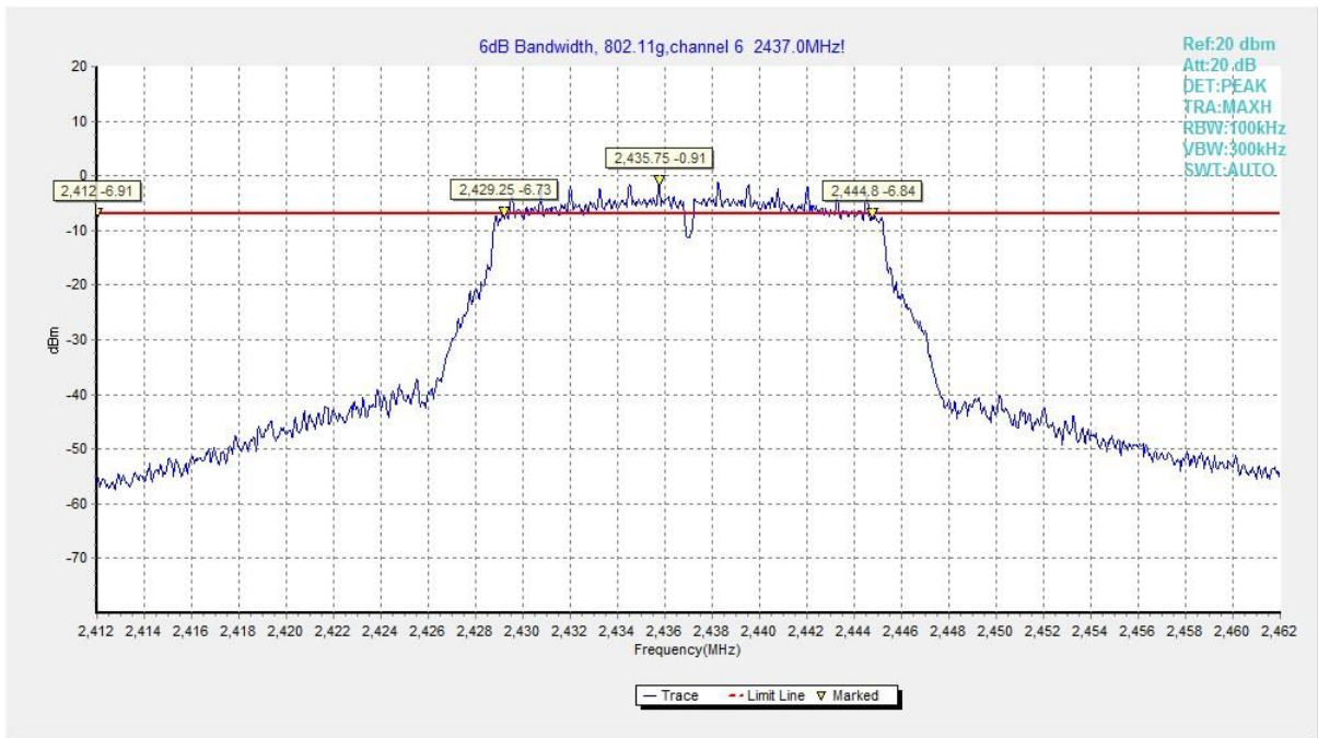
Fig.17 6dB Bandwidth (802.11g, CH 6)
