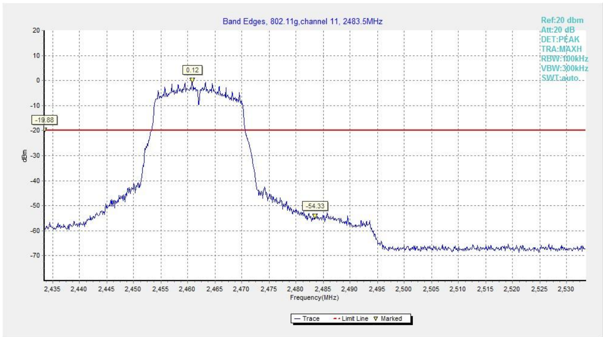
Fig.28 Band Edges (802.11g, CH 11)
