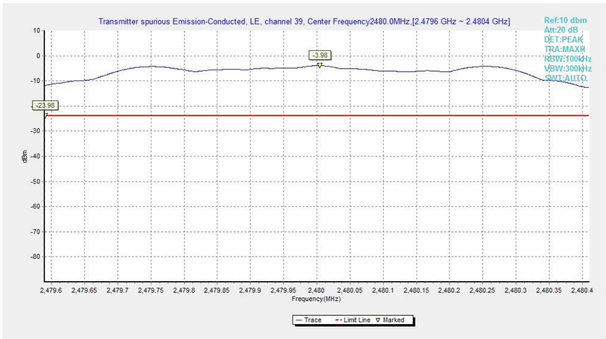
Fig.29 Conducted Spurious Emission (Ch39, Center Frequency), LE 1M
