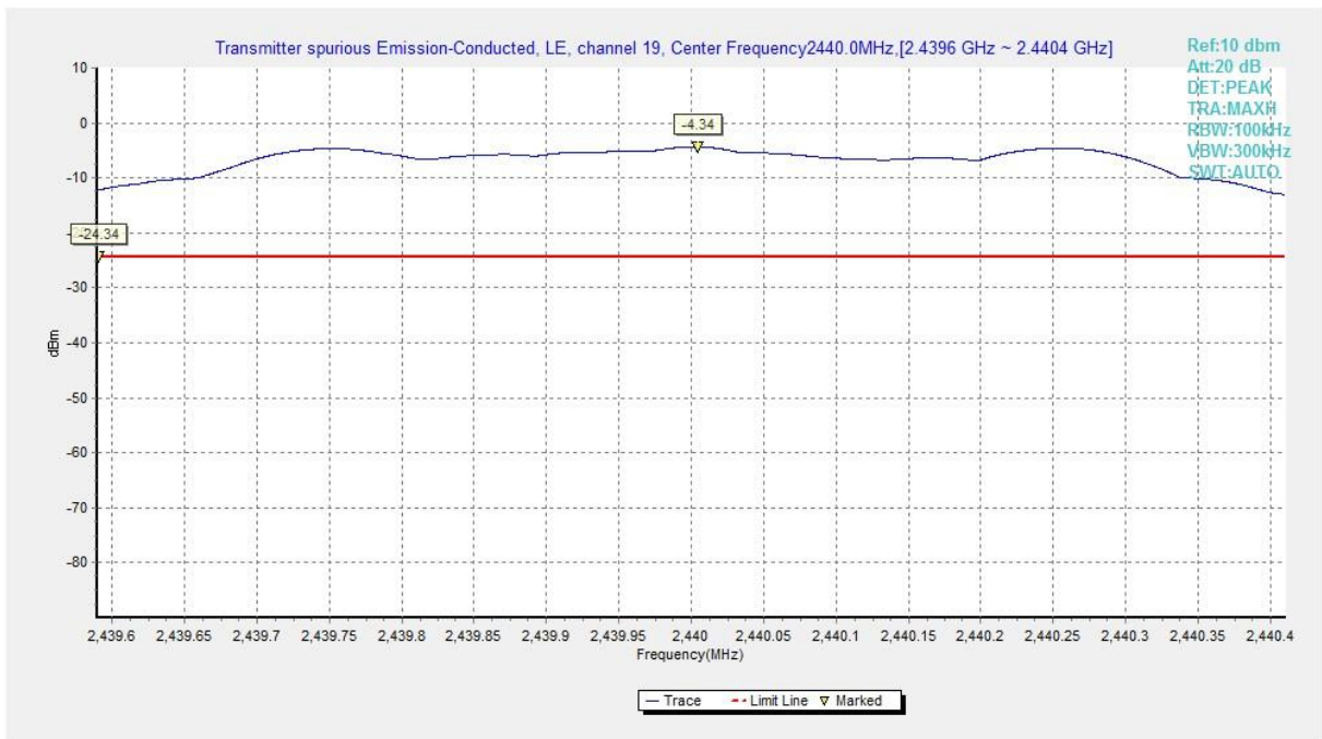
Fig.26 Conducted Spurious Emission (Ch19, Center Frequency), LE 1M
