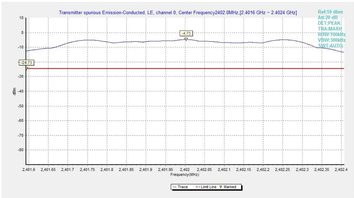
Fig.23 Conducted Spurious Emission (Ch0, Center Frequency), LE 1M
