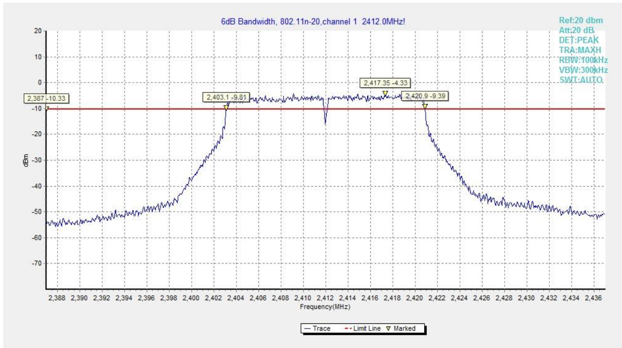
Fig.A.4.7 Occupied 6dB Bandwidth (802.11n-20MHz, Ch 1)
