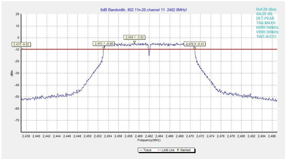
Fig.A.4.9 Occupied 6dB Bandwidth (802.11n-HT20, Ch 11)
