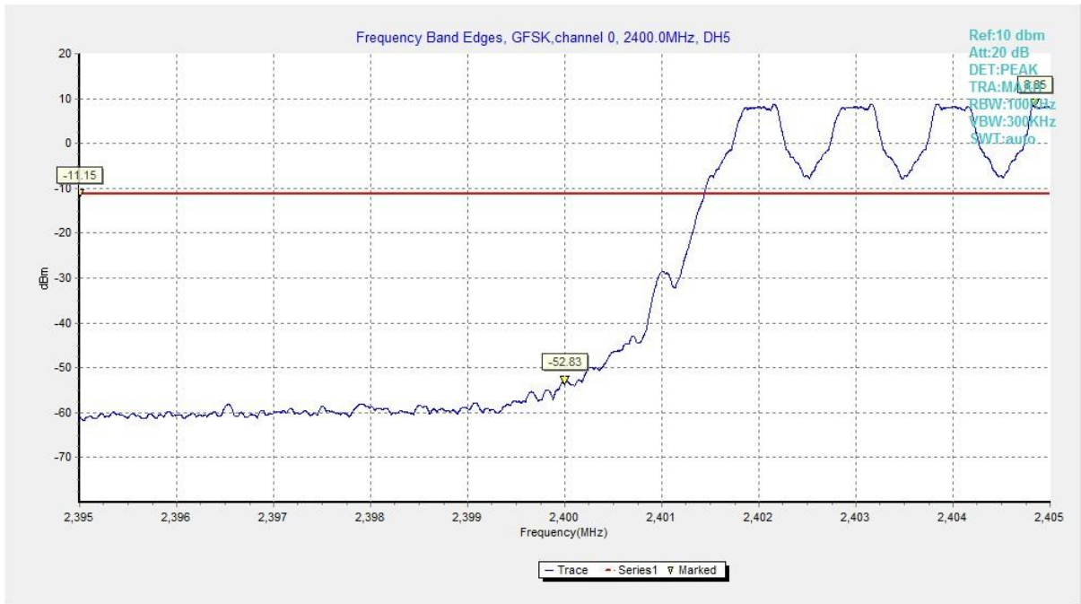
Fig. 1 Band Edges (GFSK, Ch 0, Hopping ON)
