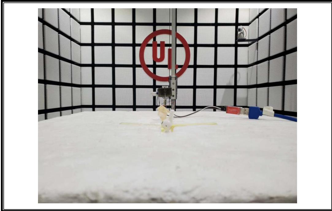
POWERLINE CONDUCTED EMISSIONS MEASUREMENT SETUP
