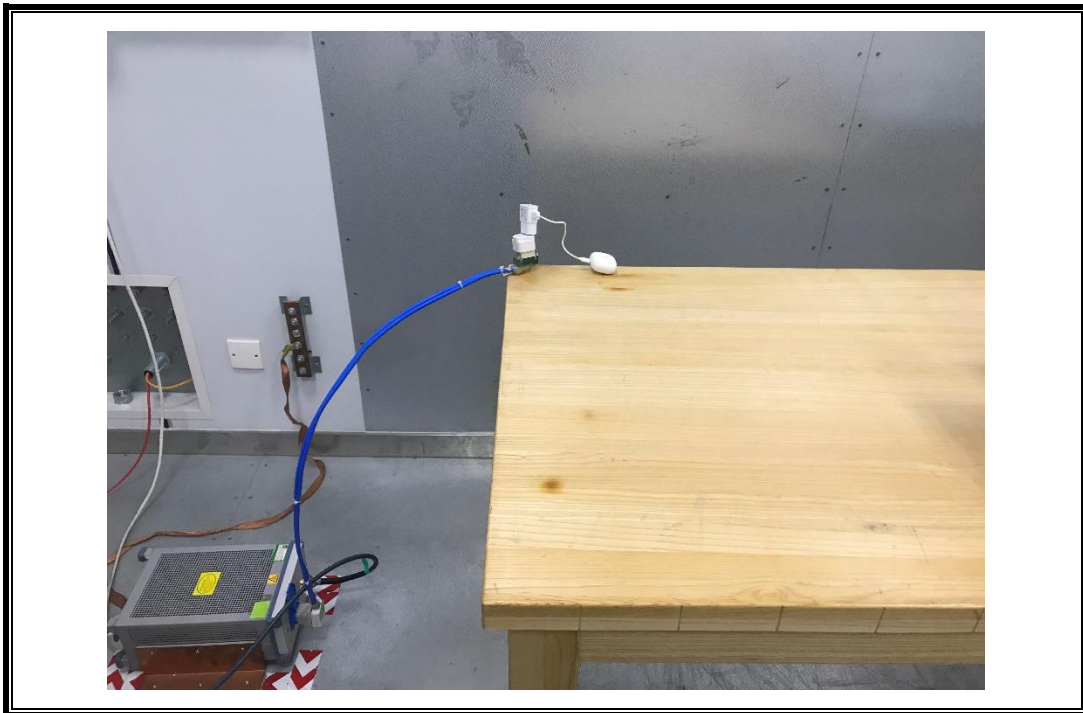
POWERLINE CONDUCTED EMISSIONS MEASUREMENT SETUP
