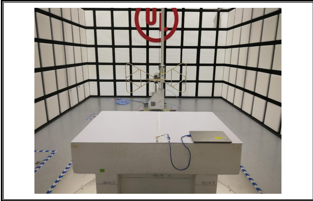
RADIATED RF MEASUREMENT SETUP (30MHz ~ 1 GHz)
