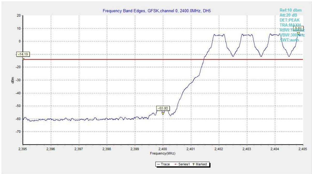
Fig. 1 Band Edges (GFSK, Ch 0, Hopping ON)
