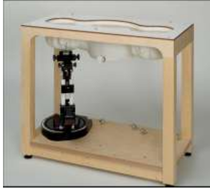
Picture C.8: SAM Twin Phantom
