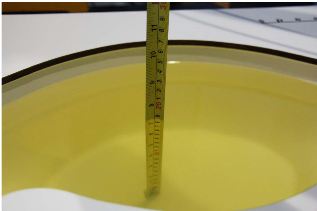
Picture 7-1: Liquid depth in the Flat Phantom(2450MHz)
