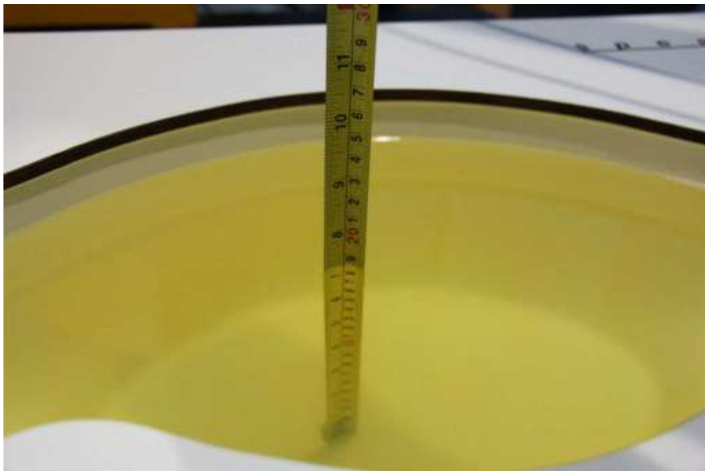
Picture 7-1: Liquid depth in the Flat Phantom(2450MHz)
