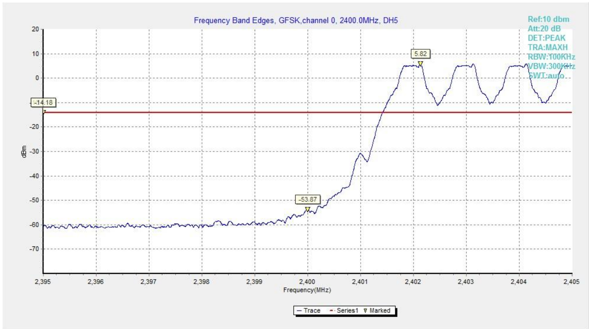
Fig. 1 Band Edges (GFSK, Ch 0, Hopping ON)
