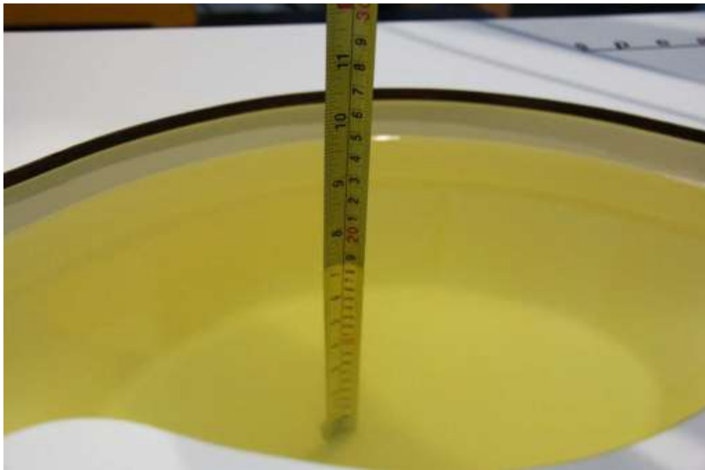
Picture 7-1: Liquid depth in the Flat Phantom(2450MHz)
