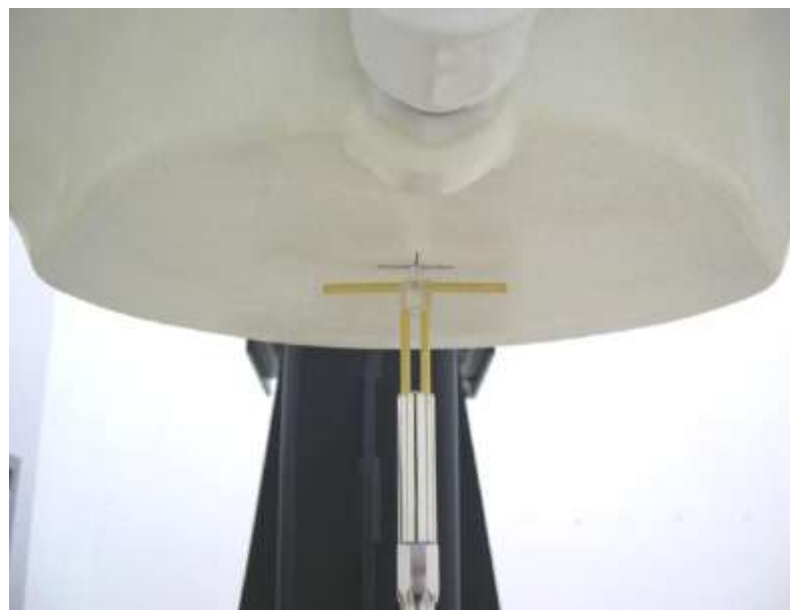
Picture 8.2 Photo of Dipole Setup
