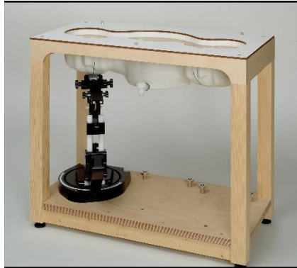
Picture C.10: SAM Twin Phantom
