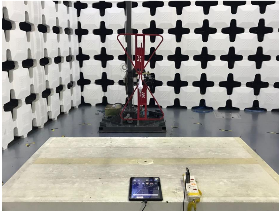
5. Radiated Emissions (Part 15B Charging Mode with Camera Mode/Video Player Mode/GSM receiver/WCDMA receiver/LTE receiver,30MHz-1GHz)
