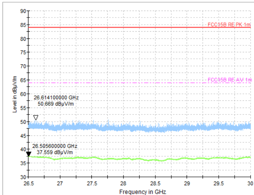
Figure A.28 Radiated Emission (Set.2, Charging and GSM850MHz idle , 26.5GHz to 30GHz)
