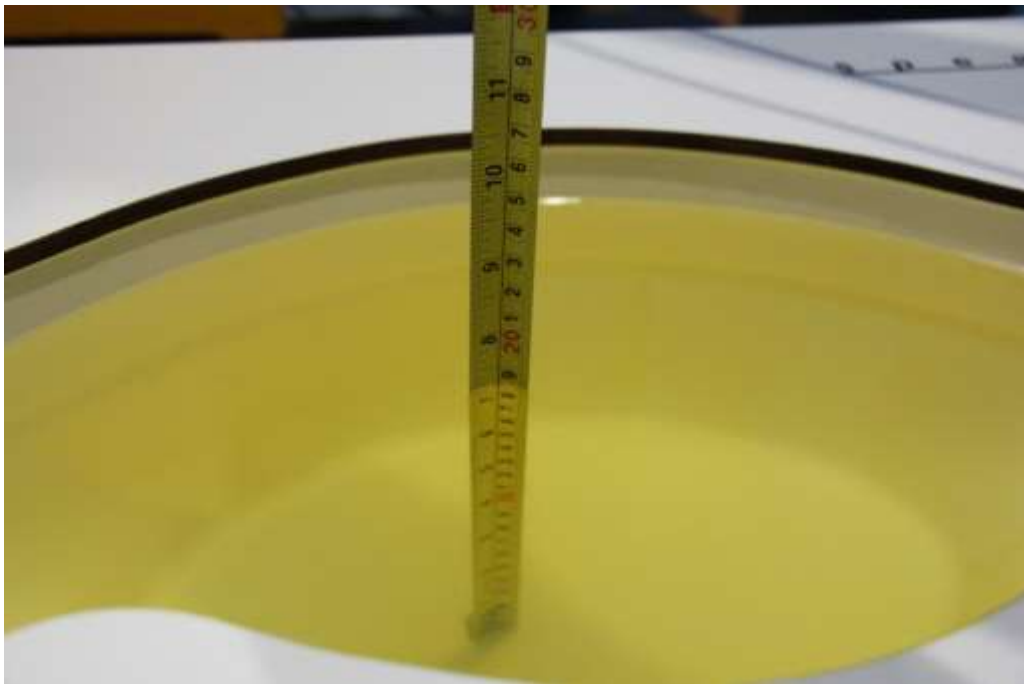
Picture 7-6: Liquid depth in the Flat Phantom(2550MHz)
