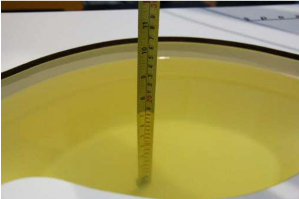
Picture 7-5: Liquid depth in the Flat Phantom(2450MHz)
