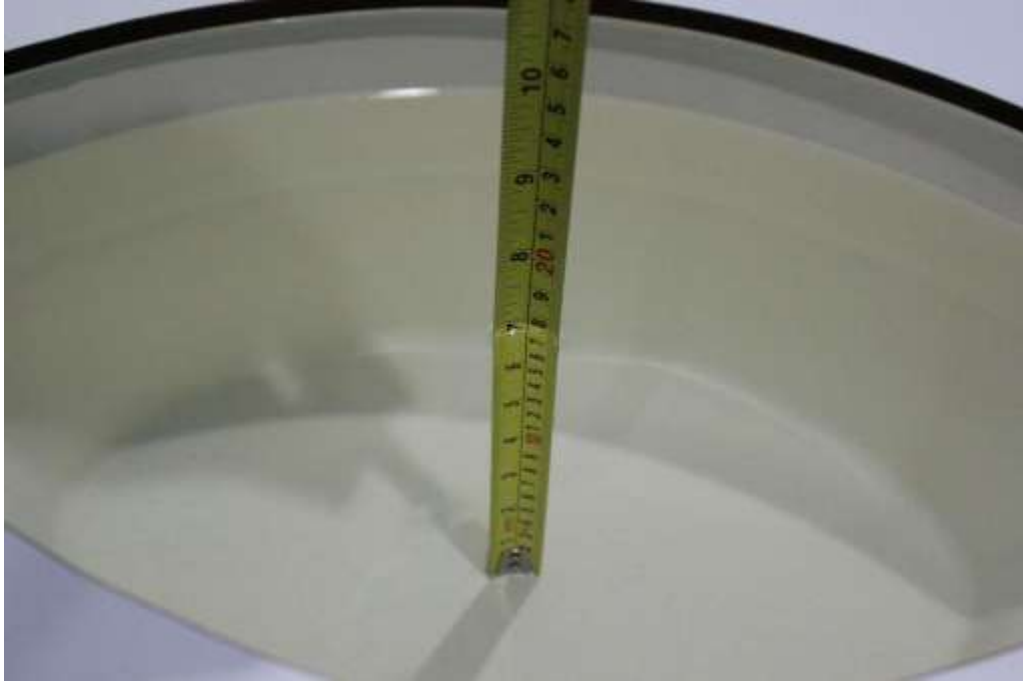
Picture 7-7: Liquid depth in the Flat Phantom(5GHz)
