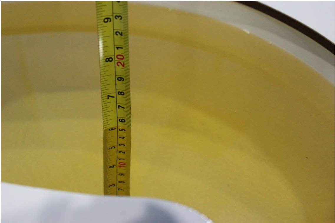
Picture 7-1 Liquid depth in the Flat Phantom (750MHz)
