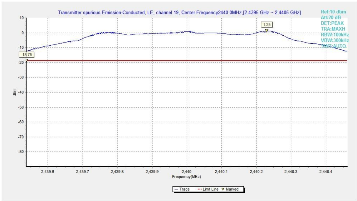
Fig.10. Transmitter Spurious Emission - Conducted: GFSK, 2440MHz
