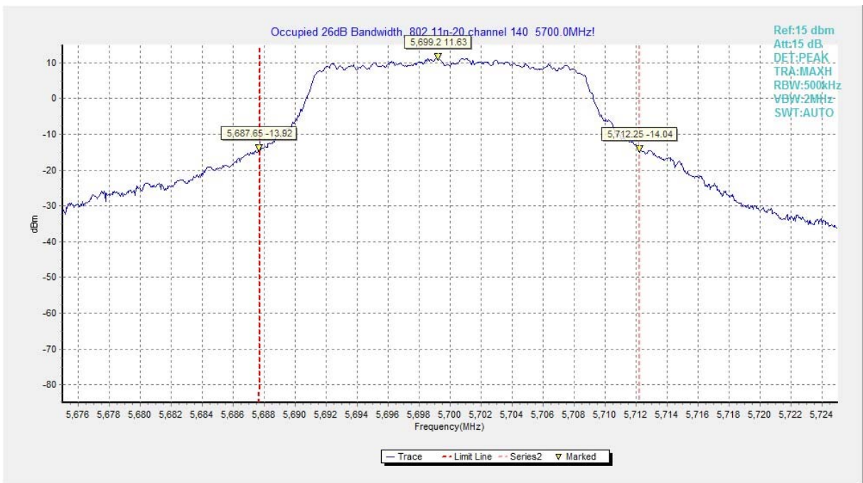
Fig.18 Occupied 26dB Bandwidth (802. 11n-HT20, 5700MHz)
