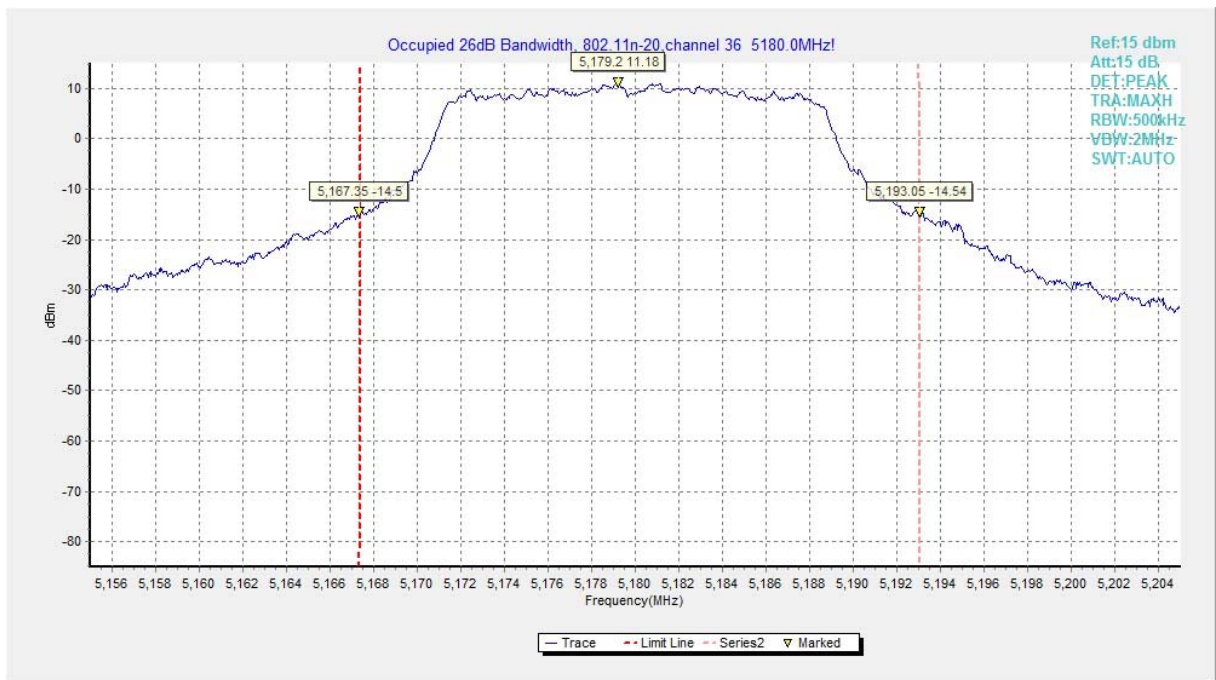
Fig.10 Occupied 26dB Bandwidth (802.11n-HT20, 5180MHz)
