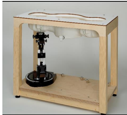
Picture C.10: SAM Twin Phantom
