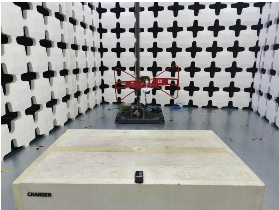
6. Radiated Emissions (Part 15C 30MHz-1GHz)
