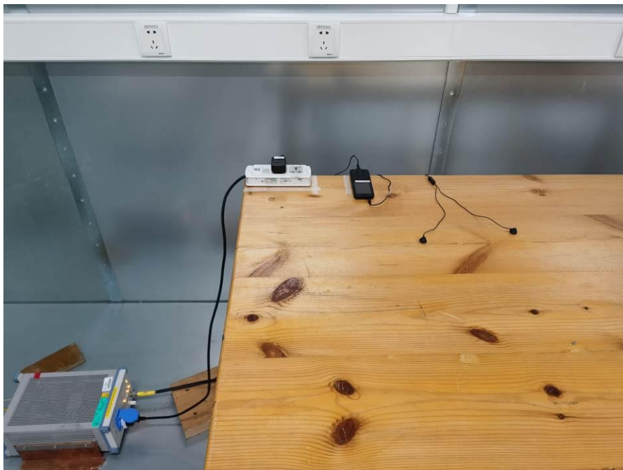
12. Conducted Emission (Part 15B, Charger mode)
