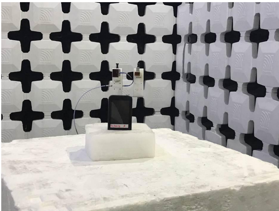
10. Radiated Emissions (Part 22/24/27, 18GHz-26.5GHz)
