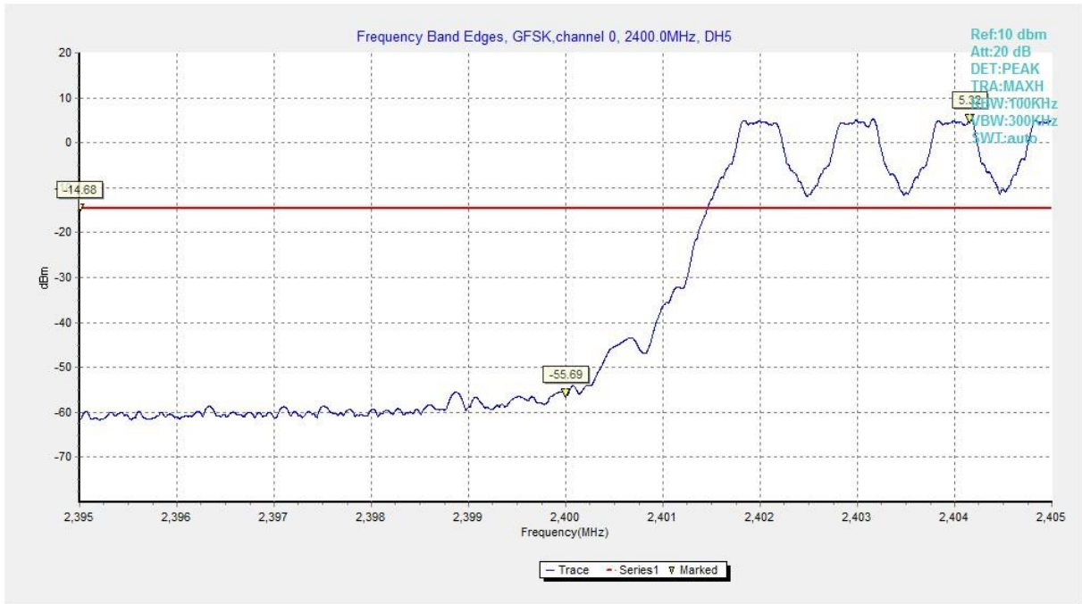
Fig. 1 Band Edges (GFSK, Ch 0, Hopping ON)
