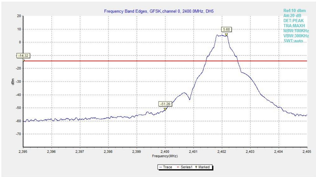
Fig. 7 Band Edges (GFSK, Ch 0, Hopping OFF)
