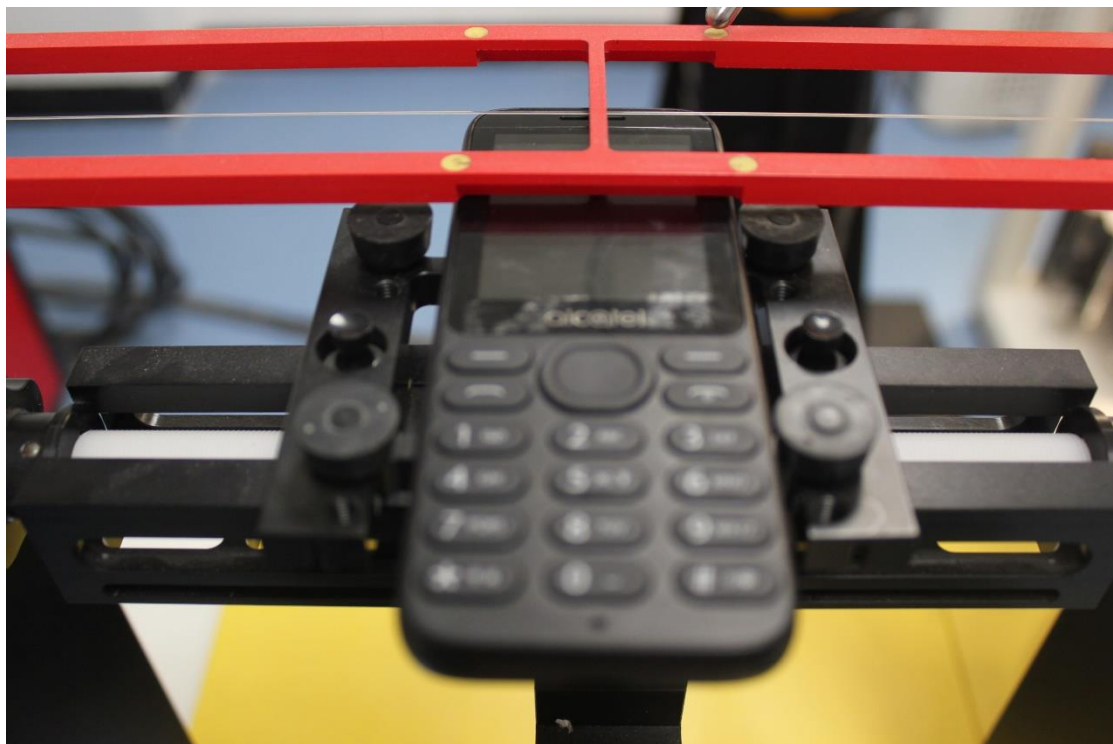
Picture 2: EUT Positioning for RF
