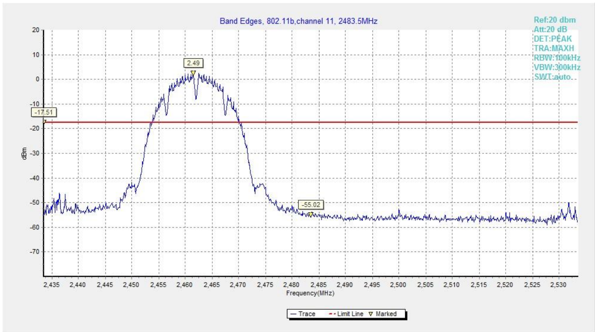
Fig.26 Band Edges (802.11b, CH 11)
