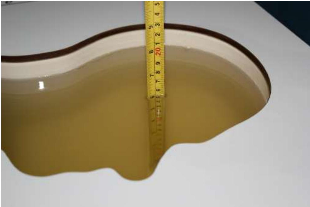
Picture 7-5: Liquid depth in the Head Phantom(2550MHz)
