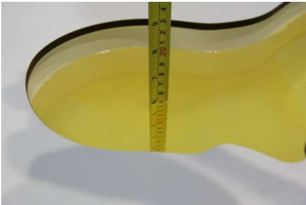
Picture 7-4: Liquid depth in the Head Phantom(2450MHz)
