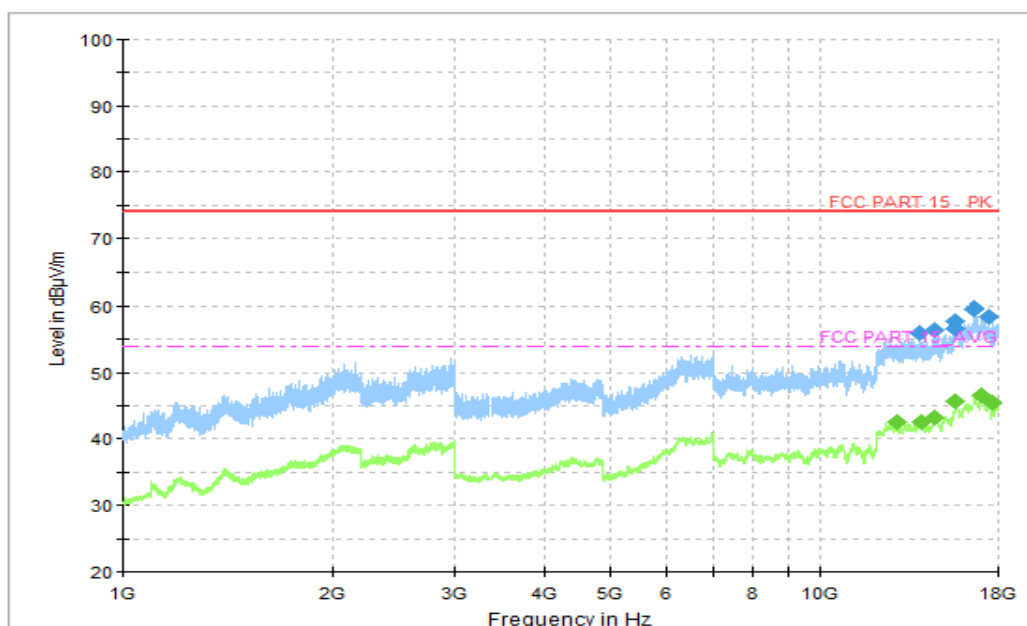
Figure A.22 Radiated Emission (Set.3, Data Transfer: PC to EUT, 1GHz to 18GHz)
