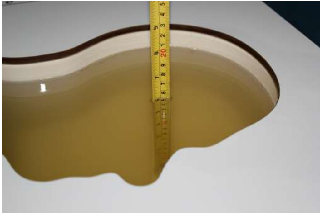
Picture 7-5: Liquid depth in the Head Phantom(2550MHz)
