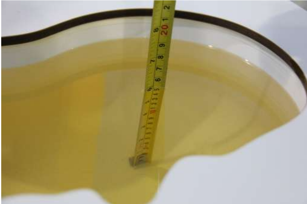
Picture 7-1: Liquid depth in the Head Phantom (835MHz)
