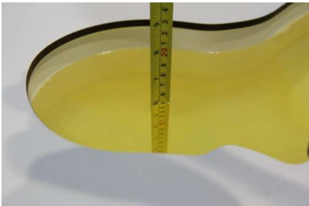
Picture 7-4: Liquid depth in the Head Phantom(2450MHz)
