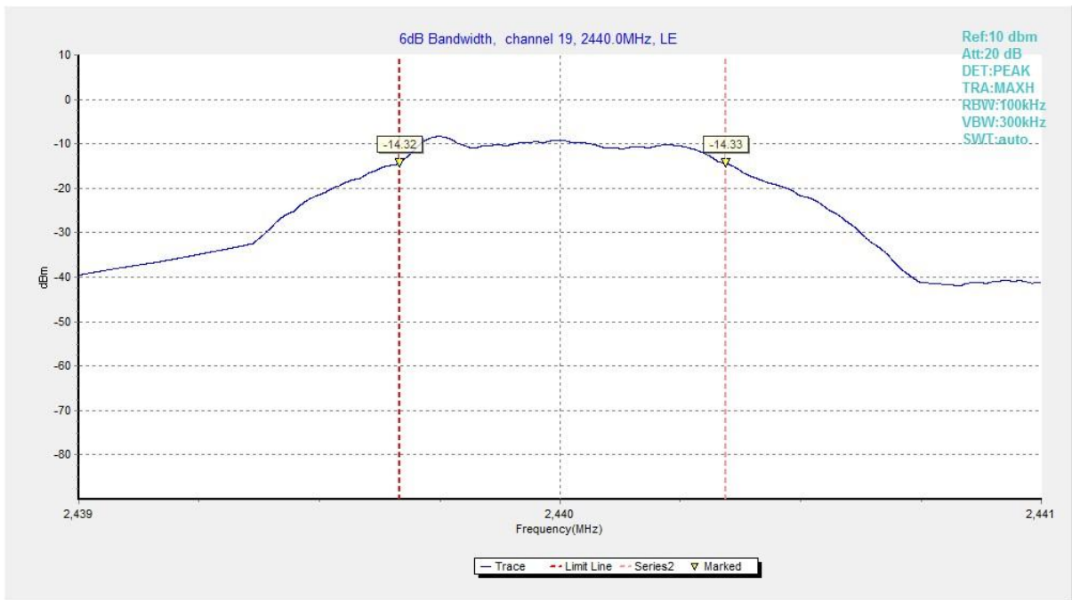
Fig.5 6dB Bandwidth (Ch 19), LE 1M
