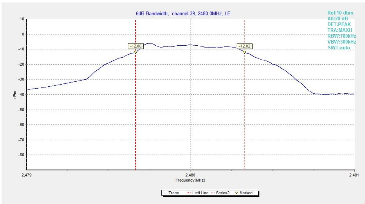
Fig.6 6dB Bandwidth (Ch 39), LE 1M
