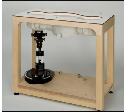
Picture C.8: SAM Twin Phantom
