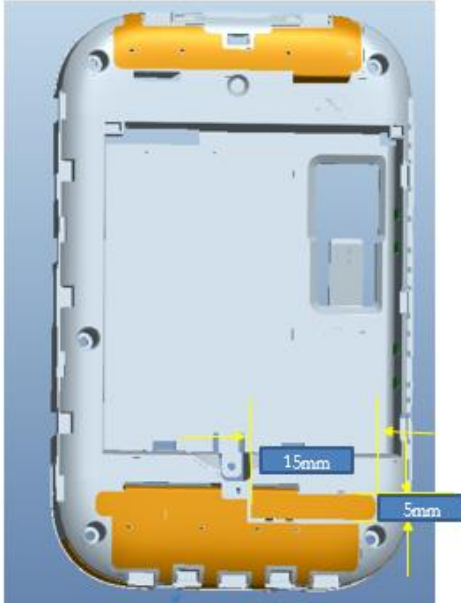
BACK side SAR Sensor Trigger Area Trigger distance :18mm
