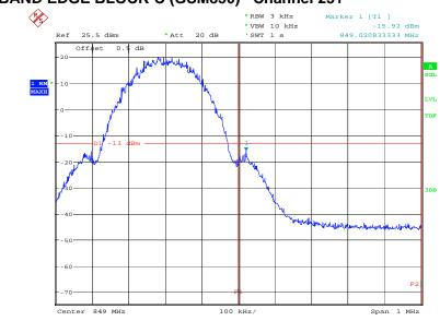
HIGH BAND EDGE BLOCK-C (GSM850) – Channel 251
