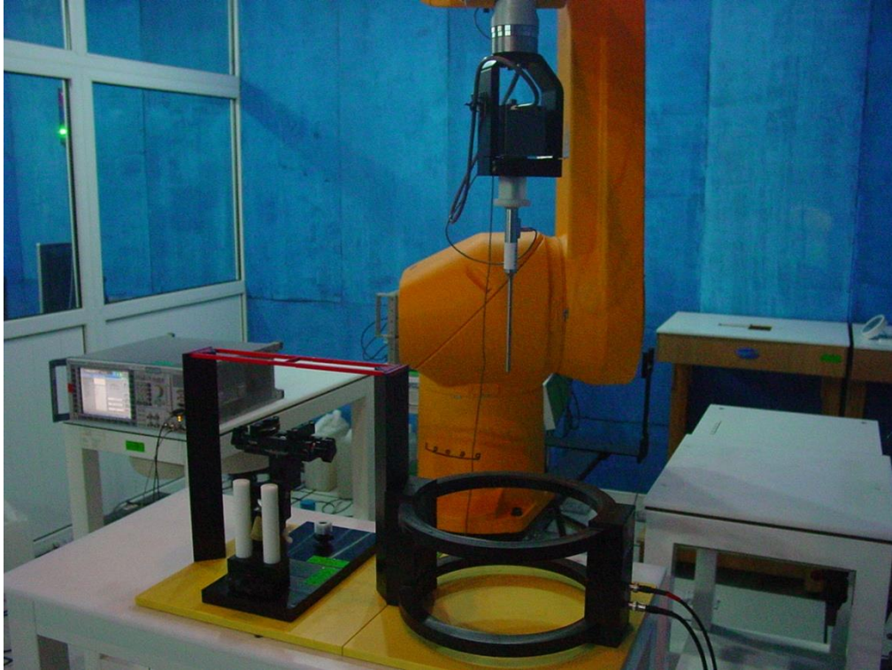
Picture A1: HAC T-Coil System Layout
