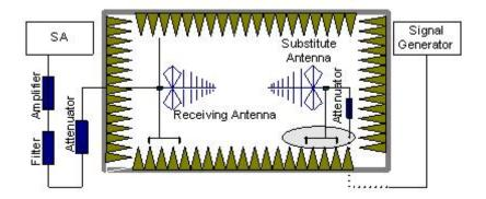
In the chamber, an substitution antenna for the frequency band of interest is placed at the reference point of the chamber. An RF Signal source for the frequency band of interest is connected to the substitution antenna with a cable that has been constructed to not interfere with the radiation pattern of the antenna. A power ( $P_{\text{Mea}}$ ) is applied to the input of the substitution antenna, and adjusts the level of the signal generator output until the value of the
