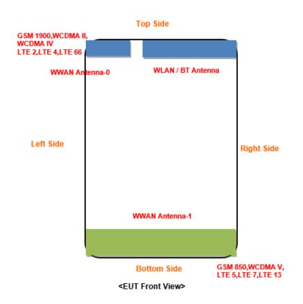
The separation distance for antenna to edge:
