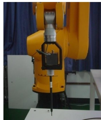
Picture C.3 E-field Probe
