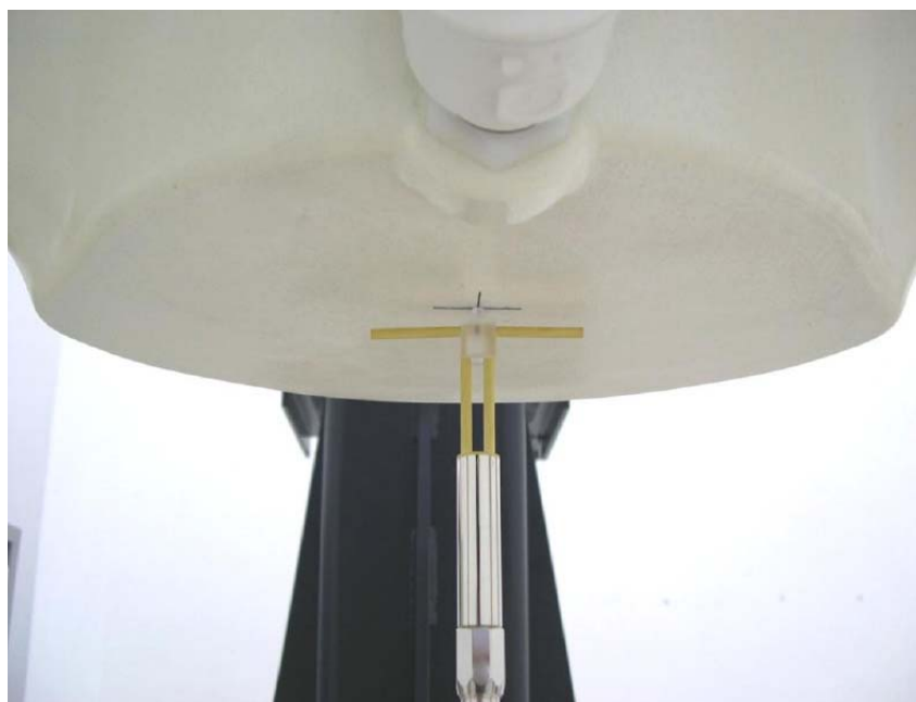
Picture 8.2 Photo of Dipole Setup
