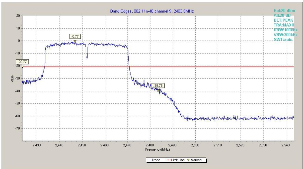
Fig.A.5.8 Band Edges (802.11n-HT40, Ch 9)
