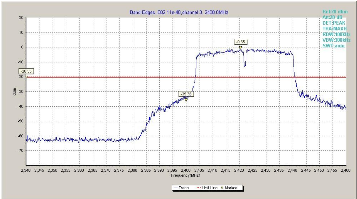
Fig.A.5.7 Band Edges (802.11n-HT40, Ch 3)
