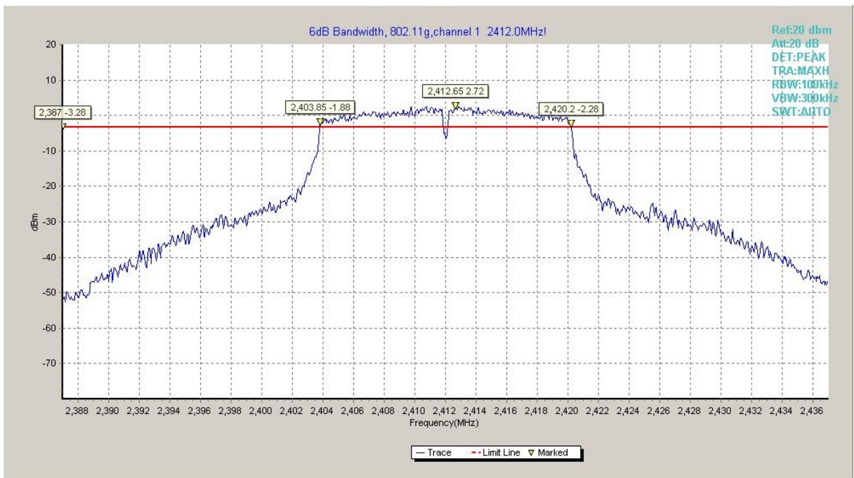
Fig.A.4.4 Occupied 6dB Bandwidth (802.11g, Ch 1)
