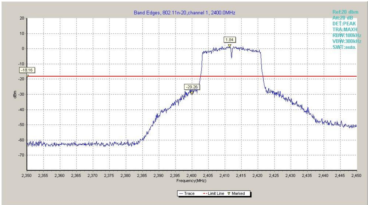
Fig.A.5.5 Band Edges (802.11n-HT20, Ch 1)
