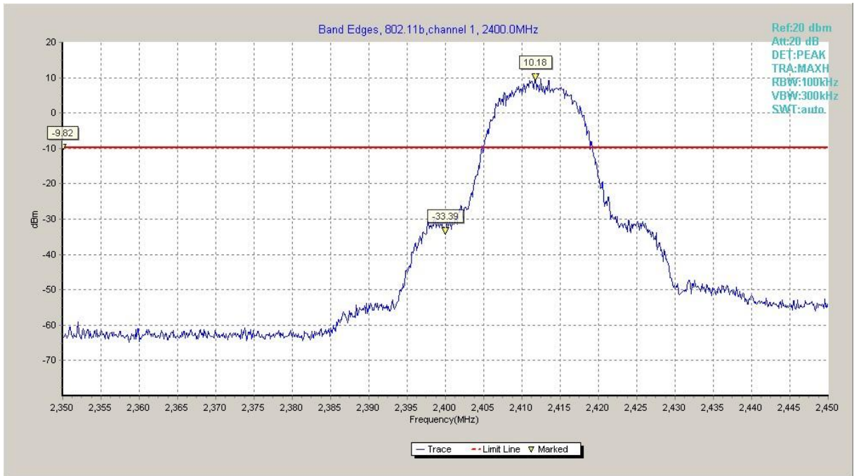
Fig.A.5.1 Band Edges (802.11b, Ch 1)
