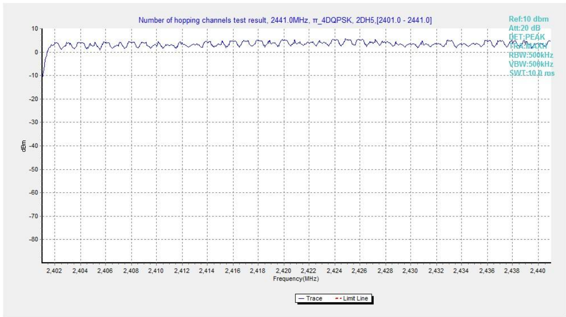
Fig.96. Number of hopping frequencies: \pi/4 DQPSK, Channel 0 - 39
