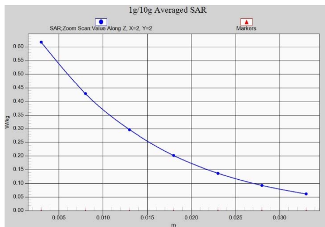
Fig.A.1- 14 Z-Scan at power reference point (LTE band4)
