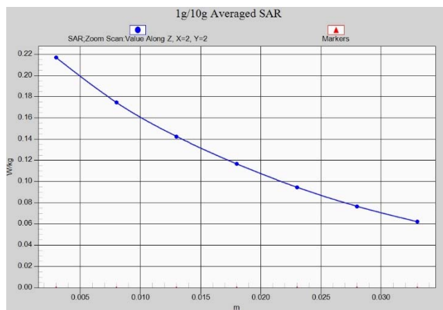
Fig.A.1- 21 Z-Scan at power reference point (LTE band13)
