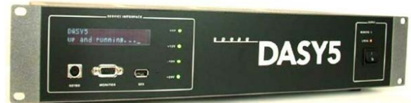
Picture C.8 Server for DASY 5
