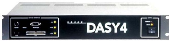
Picture C.7 Server for DASY 4
