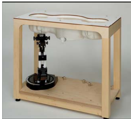
Picture C.10: SAM Twin Phantom
