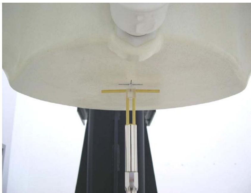
Picture 8.2 Photo of Dipole Setup
