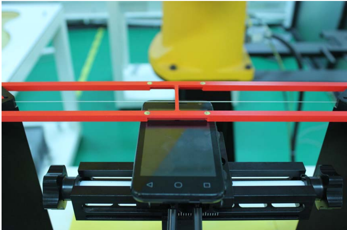
Picture 2: EUT Positioning for RF/T-coil
