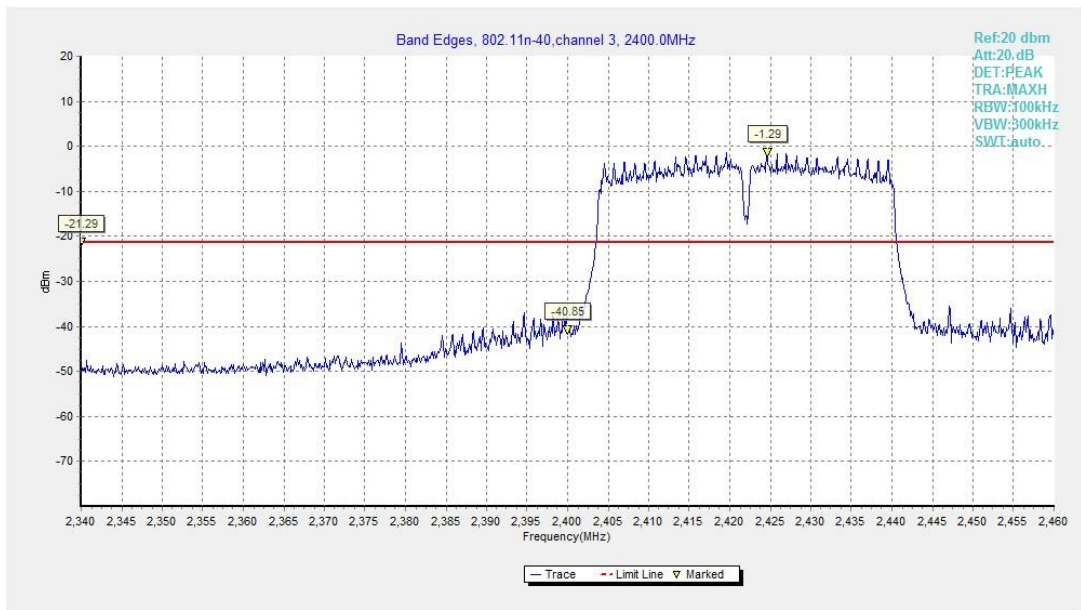
Fig.A.5.7 Band Edges (802.11n-HT40, Ch 3)
