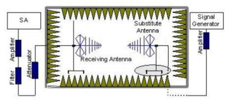
In the chamber, an substitution antenna for the frequency band of interest is placed at the reference point of the chamber. An RF Signal source for the frequency band of interest is
